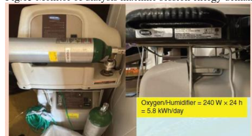
Fig.16: Oxygen and humidifier equipment requiring 5.8kWh/day.
