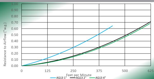
The Camfil AQ13 high-capacity pleated panel filter delivers high indoor air quality and extended service life with pressure drops suitable for most applications.
