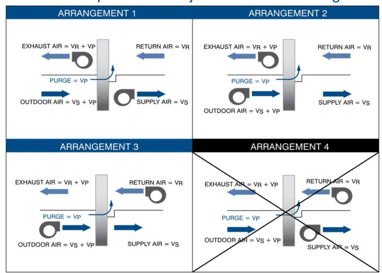
Figure 2 Fan arrangements for energy recovery exchangers
