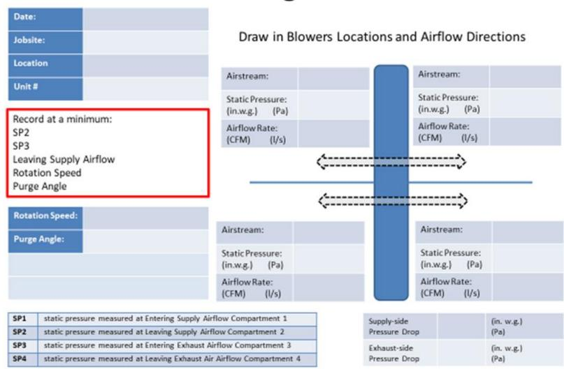
Figure 4 Field Recording Sheet for ERV Exchanger Operating Parameters
