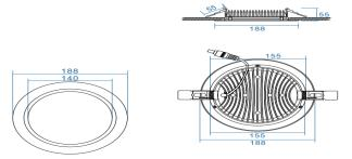
Installation: Keep a minimum 55 mm security distance between the luminaire and the ceiling to ensure its correct performance. Cutout minimum: 155mm
