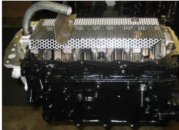
**DCR Performance Oil Pump**— The Performance Coated Oil Pump is to be torque to 20ft/lbs. For optimal performance it is Darrell Cox highly recommended that you use the DCR Pickup Tube and DCR Big Filter Kit.
