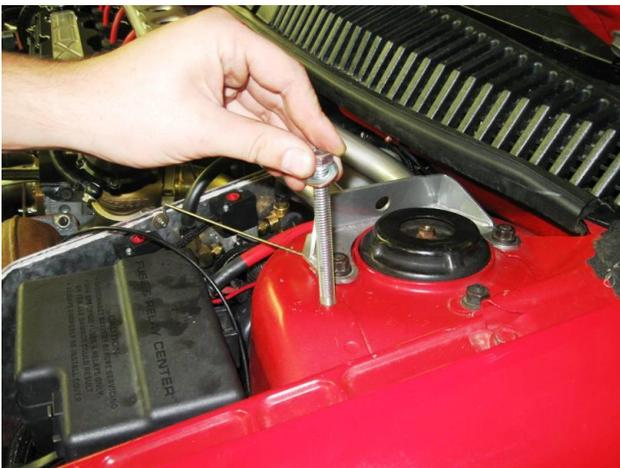
Using 1/2 inch bolt supplied with lock washer on top side as shown place thru strut tower and attach to DCR Drag Strap. Depending on ride height you may need to lower car down so control arm is compressed so that the bolt will reach the threaded coupler on upper end of drag strap.
