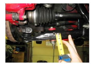
Measure 1" from bottom of a lower control arm and make a mark as shown.
