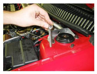
Using 1/2 inch bolt supplied with lock washer on top side as shown place thru strut tower and attach to DCR Drag Strap. Depending on ride height you may need to lower car down so control arm is compressed so that the bolt will reach the threaded coupler on upper end of drag strap.
