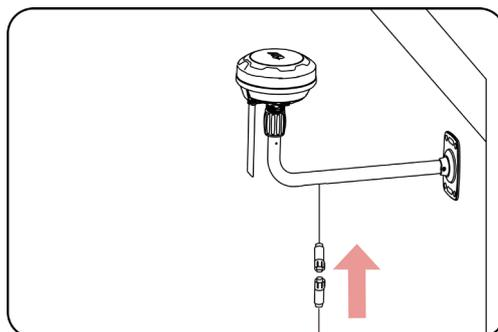
8. Connect the RTK reference station cable (10 m/33 ft.) to the RTK reference station power supply.
