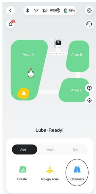
The channel is intended to connect various task areas or link the task area with charging station.
