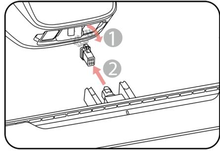
2. Place the bumper into position with the front indicator facing upwards by pressing and holding the buttons.
