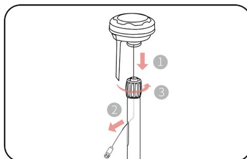
5. Secure the charging station on the flat surface using the five fixing screws. Place a gasket onto the inlet, then insert and fix the trident ground stake as shown in the figure and keep it upright.
