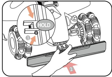
3. Install and tighten the two screws using a 2.5mm hex screwdriver.
