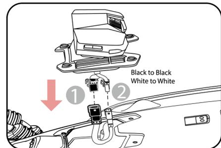
3. Attach the vision module to the Luba using the four screws and tighten them with a 2.5mm hex screwdriver.
