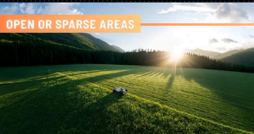
When a lawn has few visual reference points, very open spaces, or reflective surfaces, LiDAR may not provide optimal feedback. In these cases, RTK assists in positioning, improving overall accuracy and ensuring seamless mowing performance.
