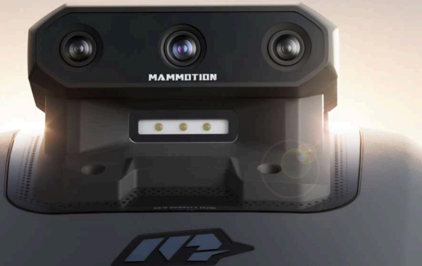
**Vision-based Navigation, using a revolutionary Tri-Camera system is present on models that do not feature LiDAR. Powered by an AI chip capable of a staggering 10 Trillion Operations Per Second. This allows the mower to act like a self-driving car, processing high-definition stereoscopic data to identify objects, plan paths, and adjust to environmental conditions in milliseconds.**
