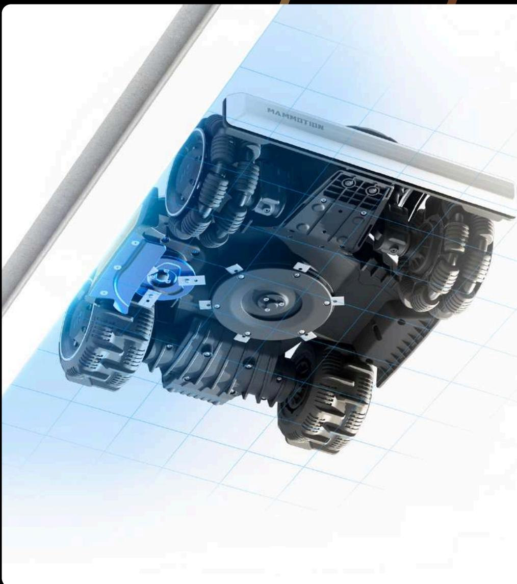
When mowing along edges where one side is lawn and the other is a different surface (e.g., a stone path or pavement), the side blade rides on the different surface to deliver a clean, precise cut along the boundary.
