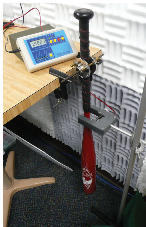
Fig. 4. Apparatus for measuring the period of oscillation for a softball bat pivoted about a point 6-in from the end of the handle.
