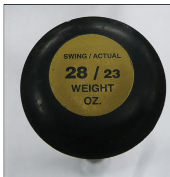
Fig. 1. The knob of a 1997 Dudley Fusion slow-pitch softball bat listing both the swing weight and the actual weight.
