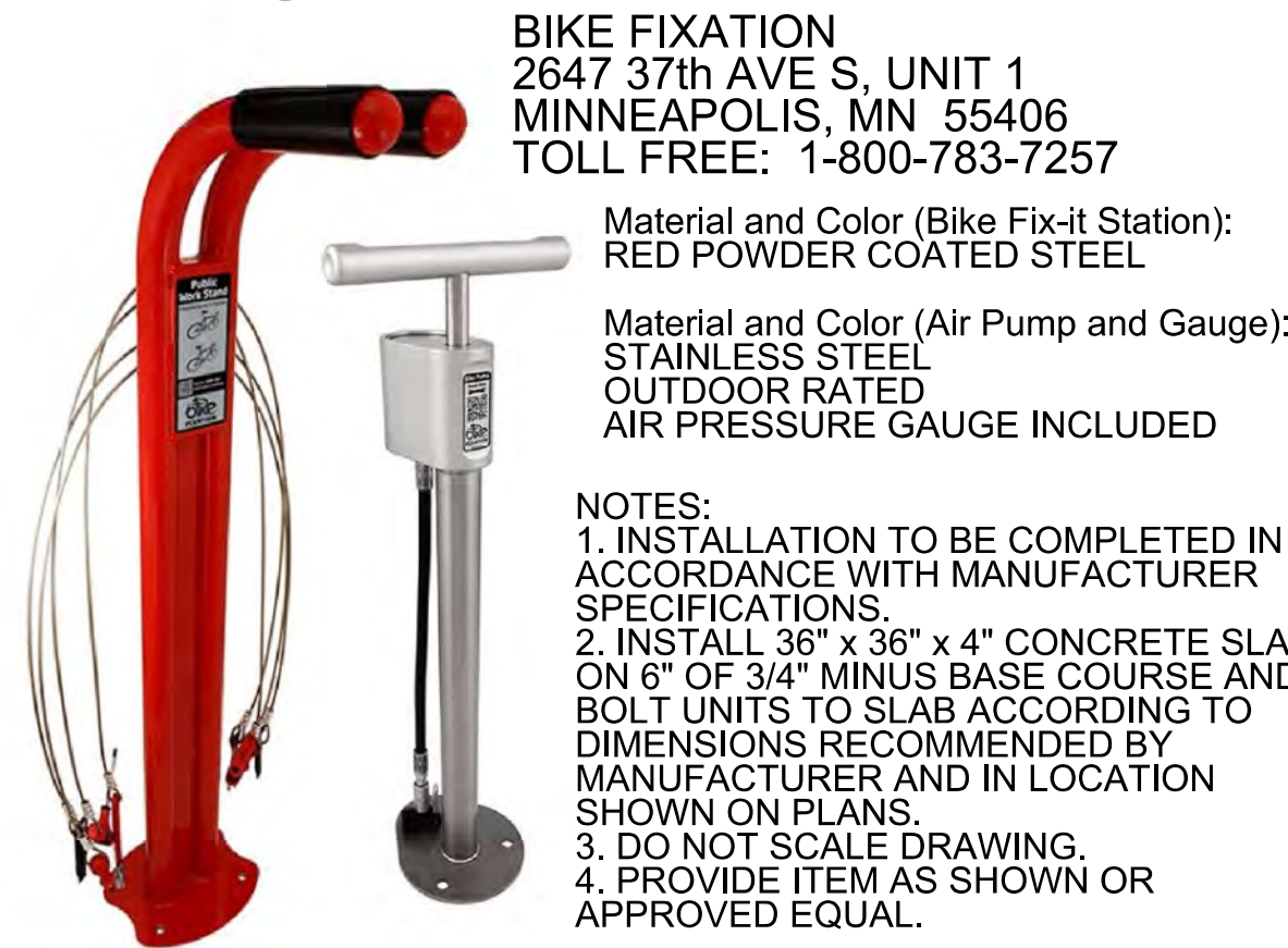
8 TYPICAL DETAIL: BIKE FIX-IT STATION 9
