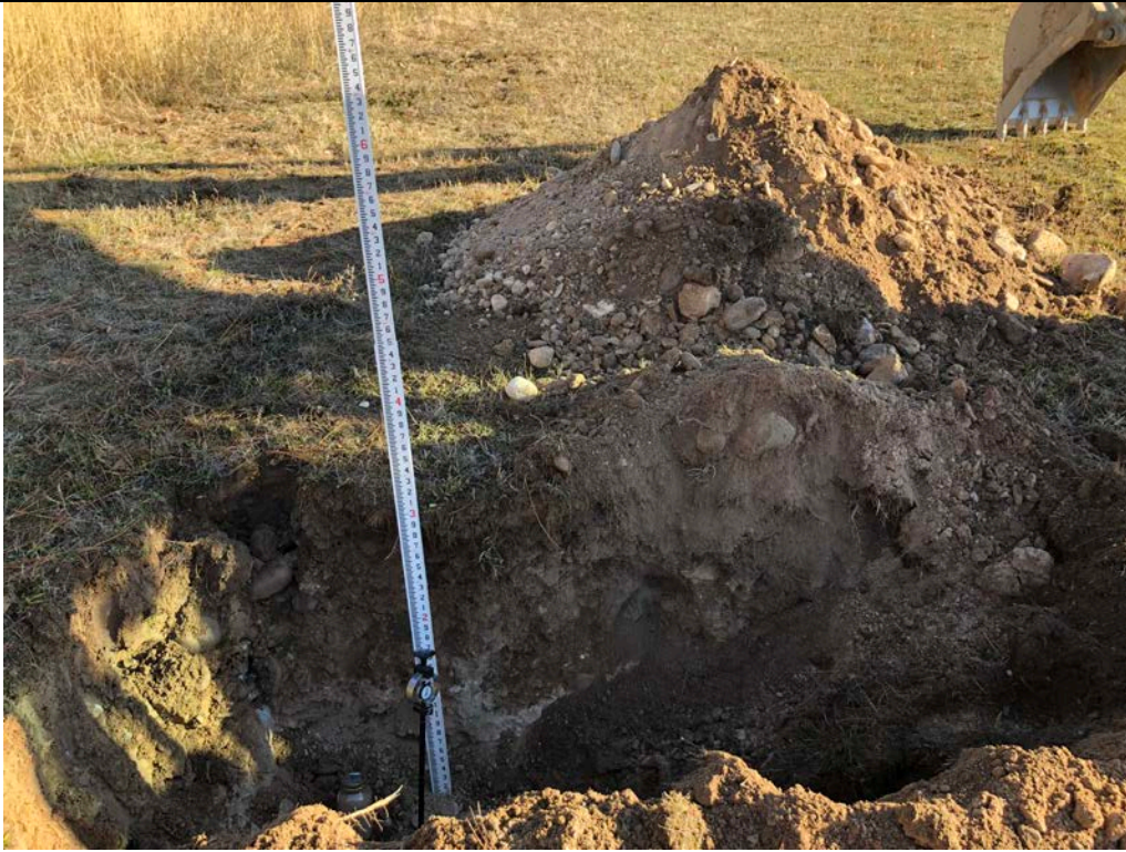
Description: TP-03 Cone Penetrometer pushed to 0.3 inches under a 320 psi loading.
