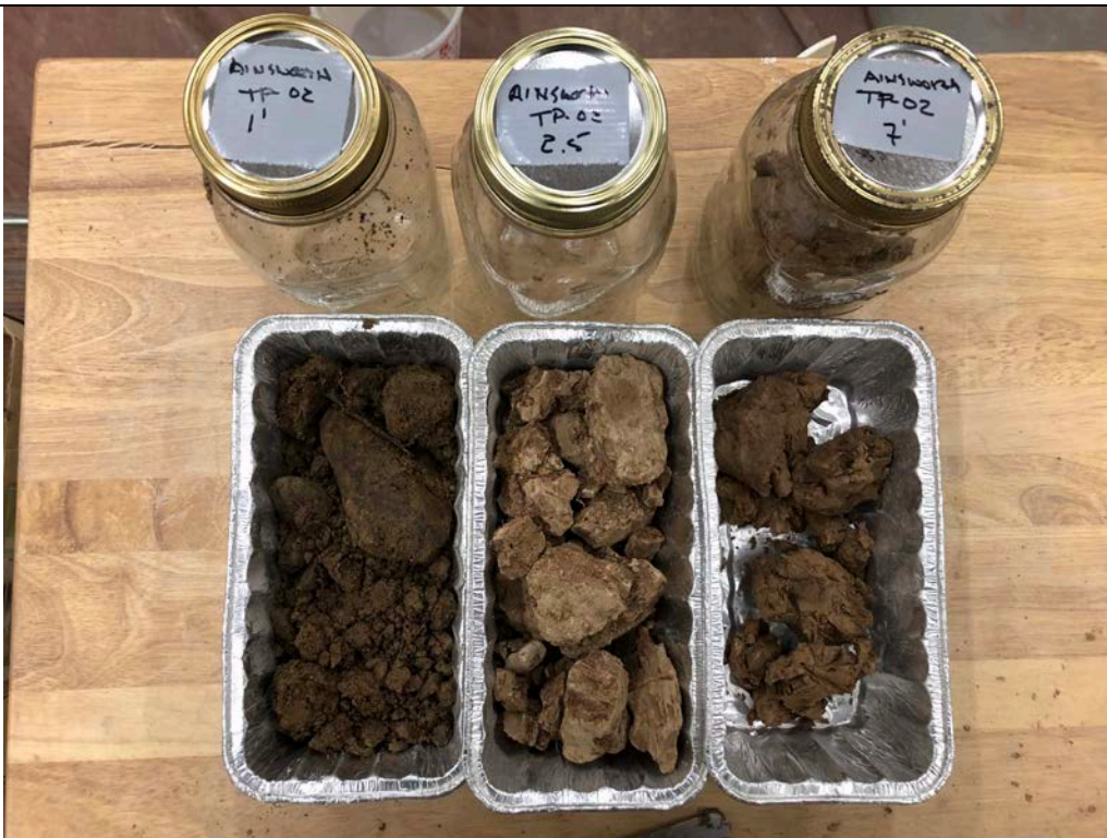
Description: TP-02 Moisture content sample prior to being placed in the drying oven.
