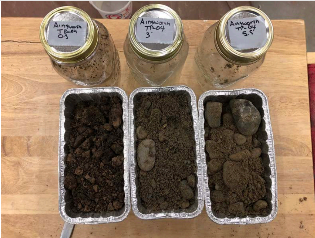
Description: TP-04 Moisture content sample prior to being placed in the drying oven.
