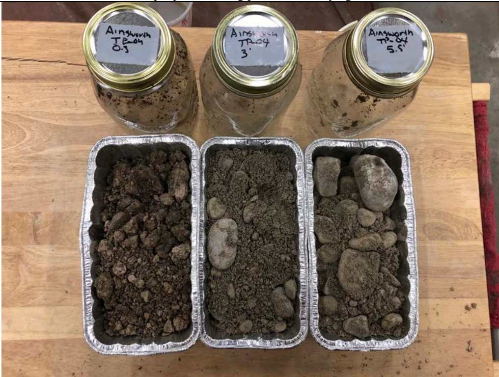
Description: TP-04 Moisture content sample after being taken out of the drying oven.
