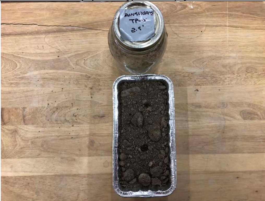
Description: TP-01 Moisture content sample after being taken out of the drying oven.
