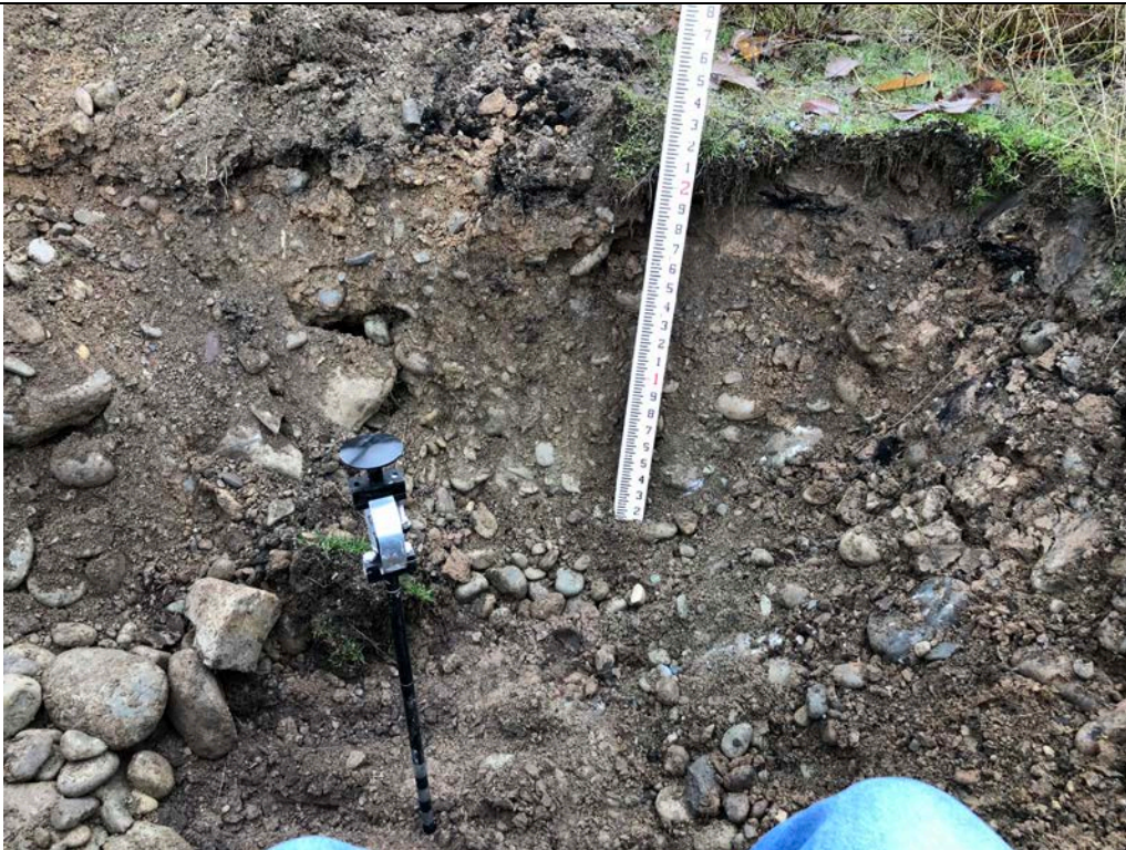
Description: TP-01 Excavated to 2.5 feet. Army Corps of Engineers Cone Penetrometer pushed to 2 inches under a 320 psi loading.
