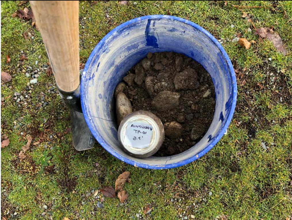
Description: TP-01 Jar sample from the 2.5-foot depth and a bulk sample from 0.5 to 2 feet.
