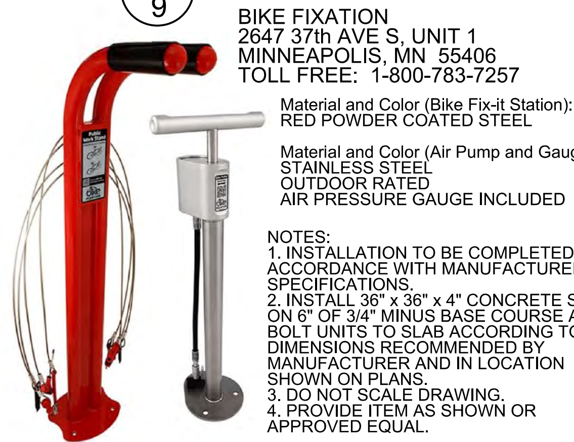
8 TYPICAL DETAIL: BIKE FIX-IT STATION 9
