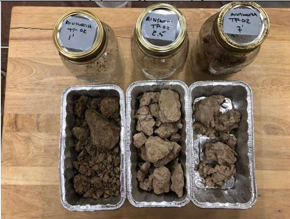
Description: TP-02 Moisture content sample after being taken out of the drying oven.
