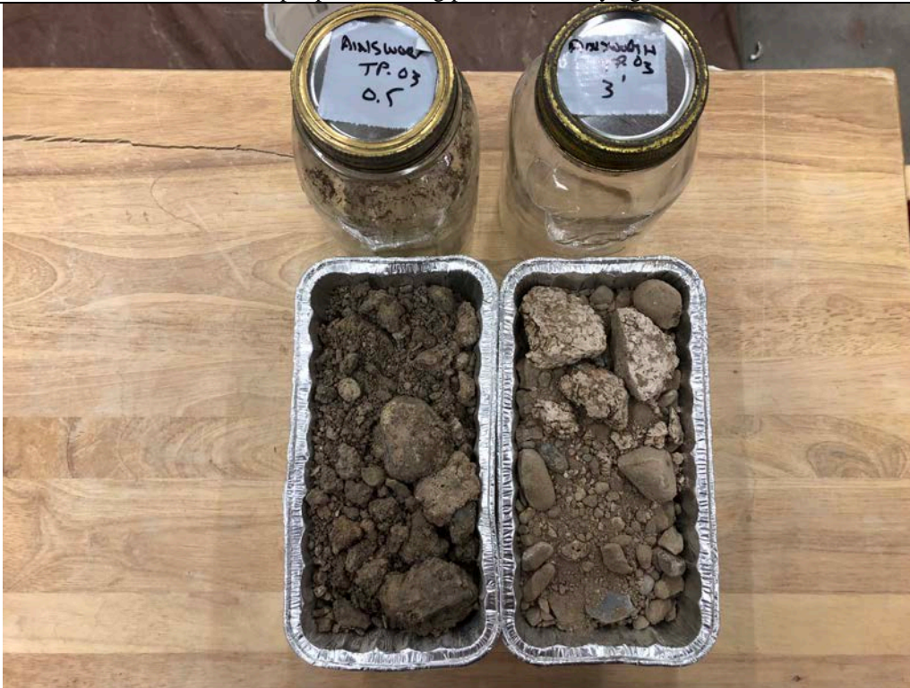
Description: TP-03 Moisture content sample after being taken out of the drying oven.
