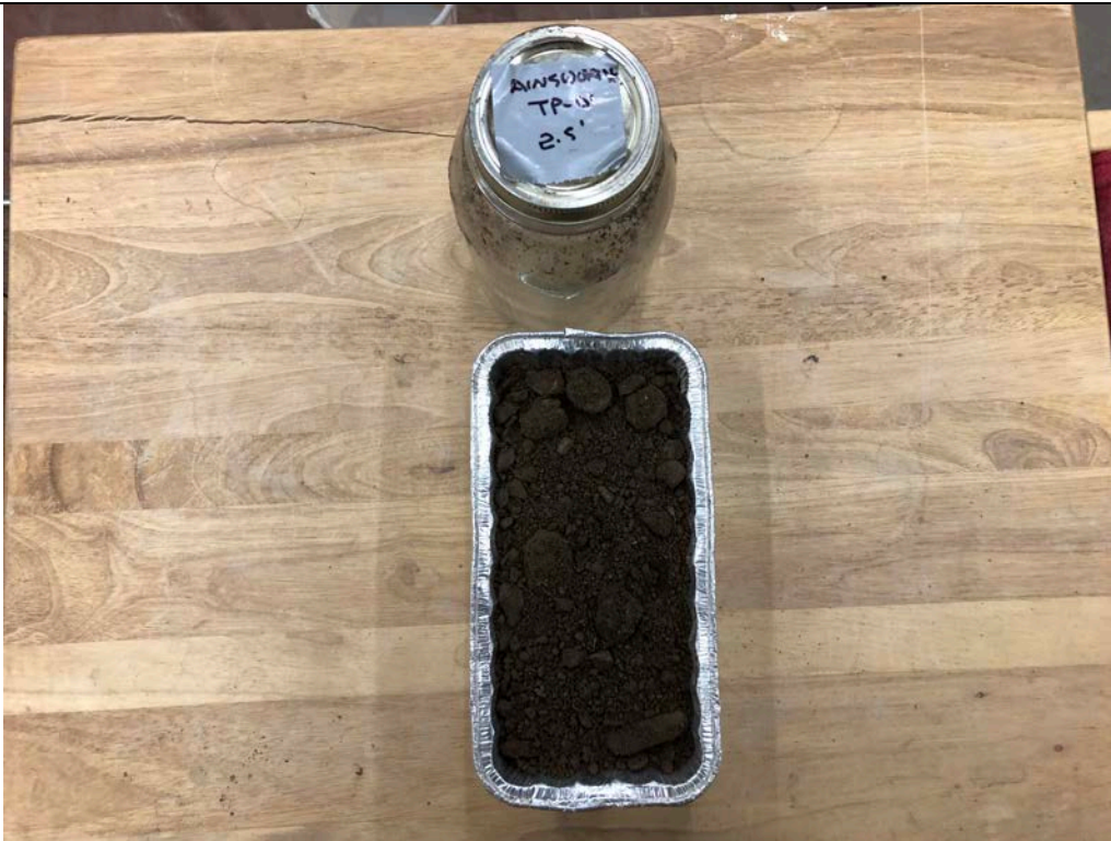
Description: TP-01 Moisture content sample prior to being placed in the drying oven.
