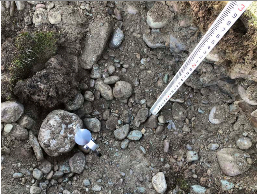
Description: TP-04 Cone Penetrometer pushed to 1 inch under a 320 psi loading.
