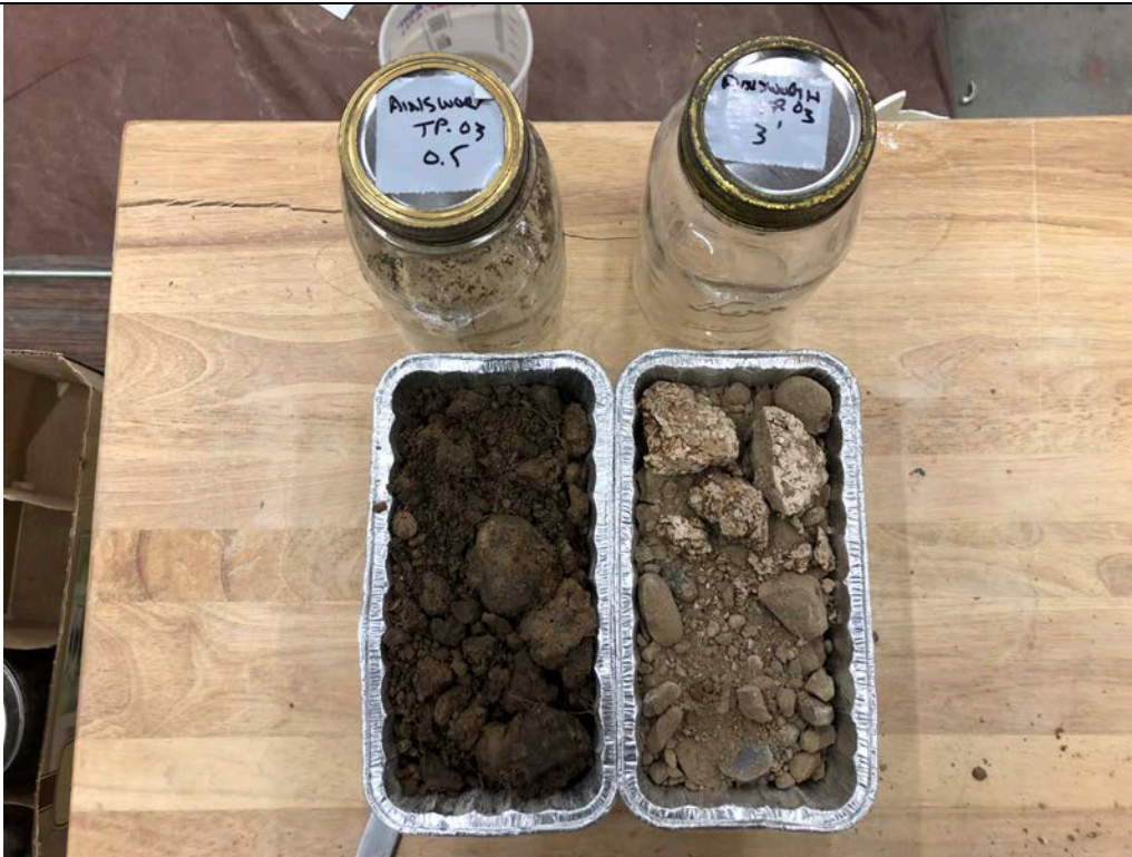
Description: TP-03 Moisture content sample prior to being placed in the drying oven.
