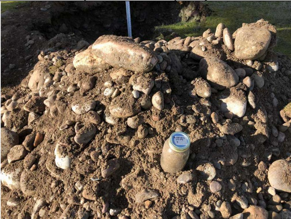
Description: TP-04 Jar sample from 3-foot depth on the spoils pile.
