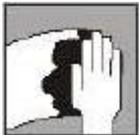
Remove wax, silicon or other contaminations with 3910 degreaser.
