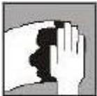
Remove wax, silicon or other contaminations with 3910 degreaser.
