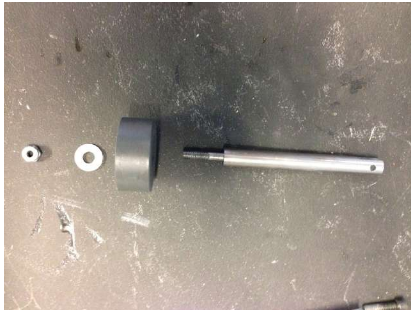
Image 44: Piston Assembly (Exploded View)
