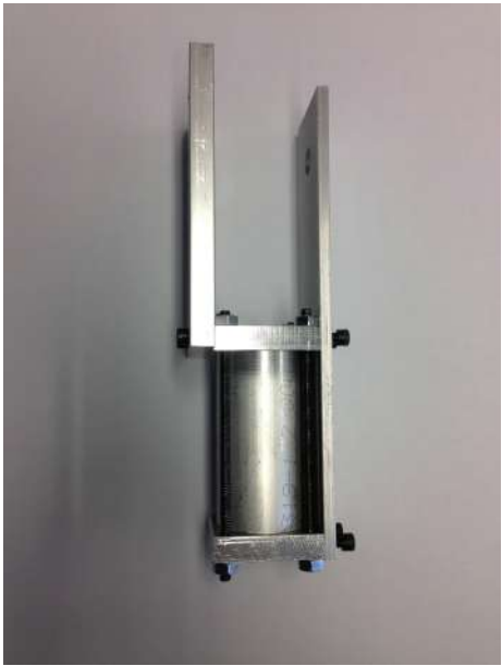
Image 29: Pump Assembly to Check hole geometry
