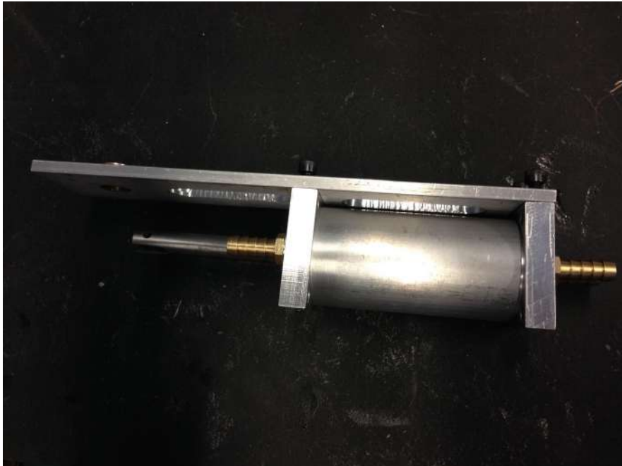
Image 50: Back Mount Plate and Piston Cylinder Assembly
