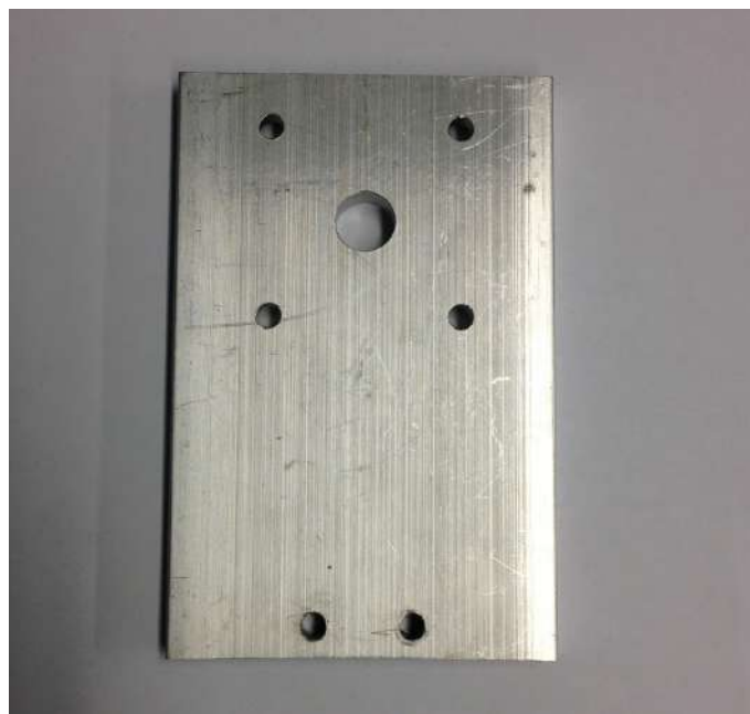
Image 32: End Caps (Left we machined the holes, right was pre machined)
