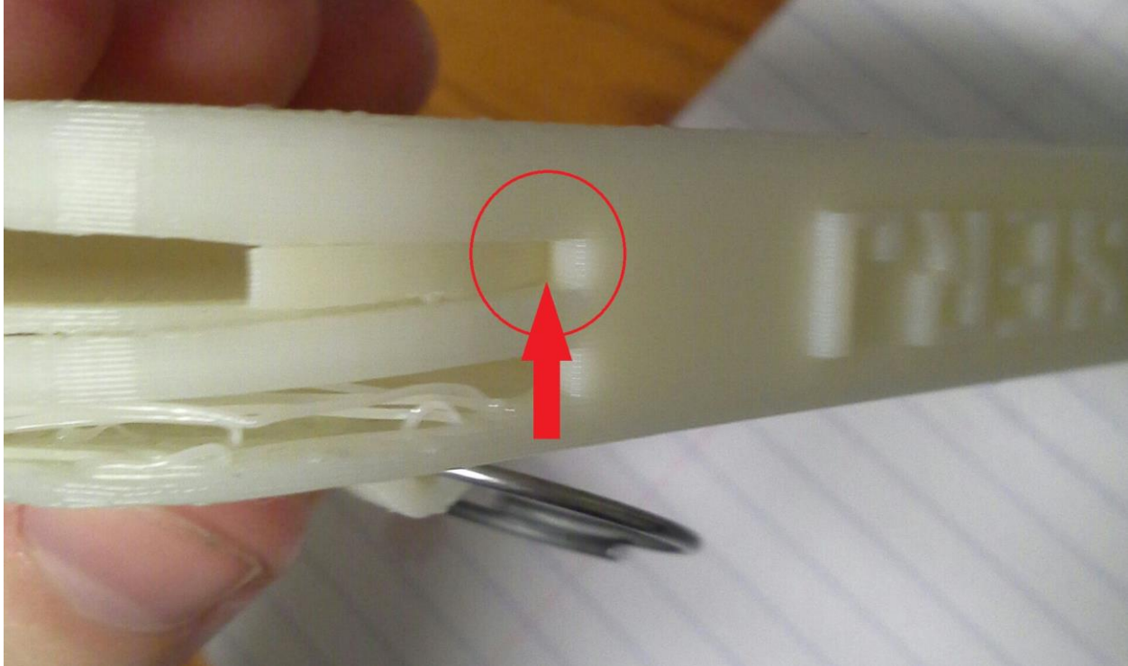
Figure 4.1: Prototype 1 image: Here, the red arrow points to where the tab runs up against the edge of the spine, and is unable to fit inside.
