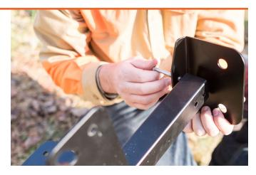
Tight the hardware on the feet so the lock nut is snug, but doesn't prevent movement as the legs are leveled up.
