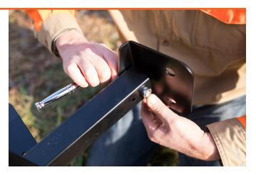
Find the two legs that are setup for the ladder bracket and position them like this on each side of the widest side of your 360 tower floor.
