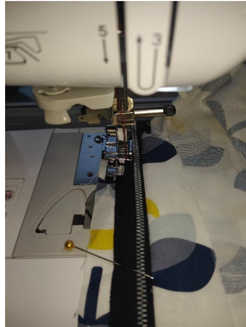
12. Adjust zipper foot to proper side of zipper tape and sew.
