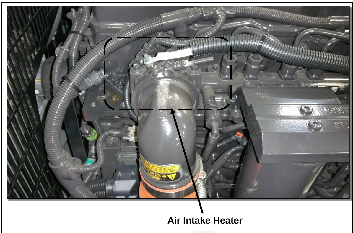
Figure 1-1-6: Air Intake Heater
