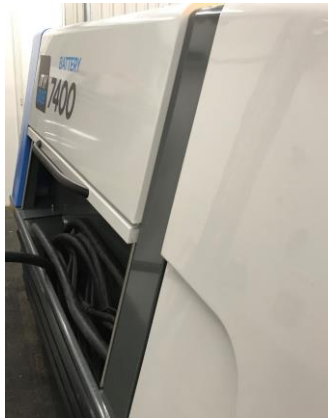
Fig 3.2.1a Cable Compartment, 50/60 Hz (open)
