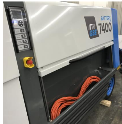
Fig 3.2.2a Cable Compartment, 400 Hz (open)
