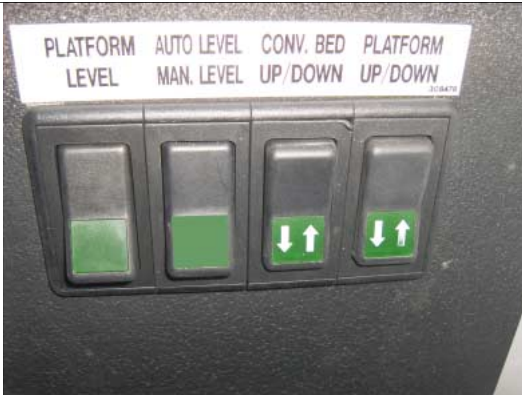
FIGURE 1-2-3. CONVEYOR PLATFORM AND LEVELING CONTROLS
