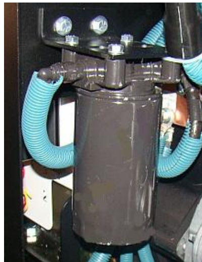
Figure 5: Primary Fuel Filter
