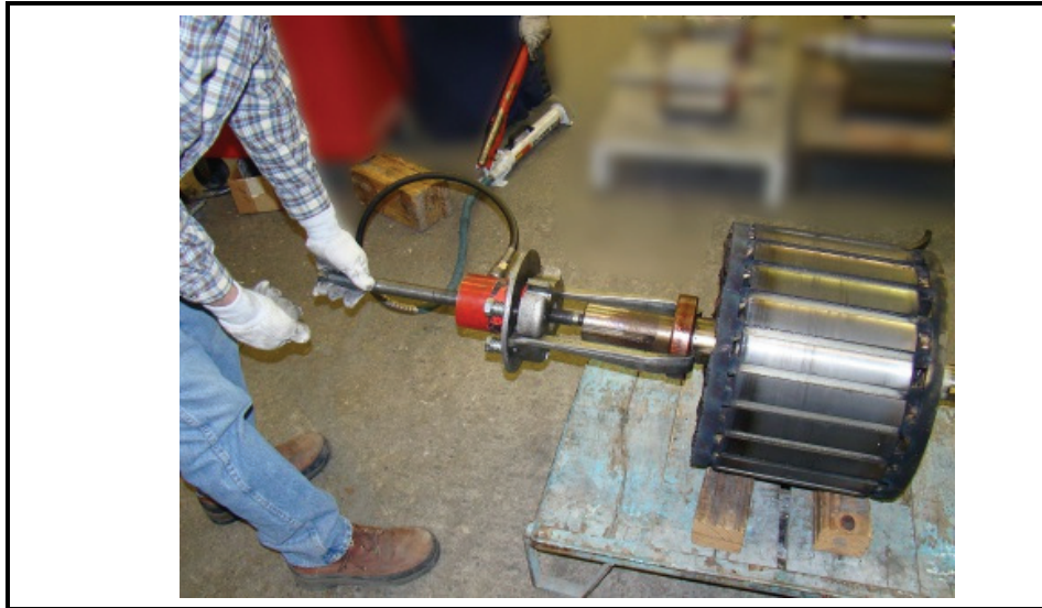
Figure 16: Removing the Bearings
