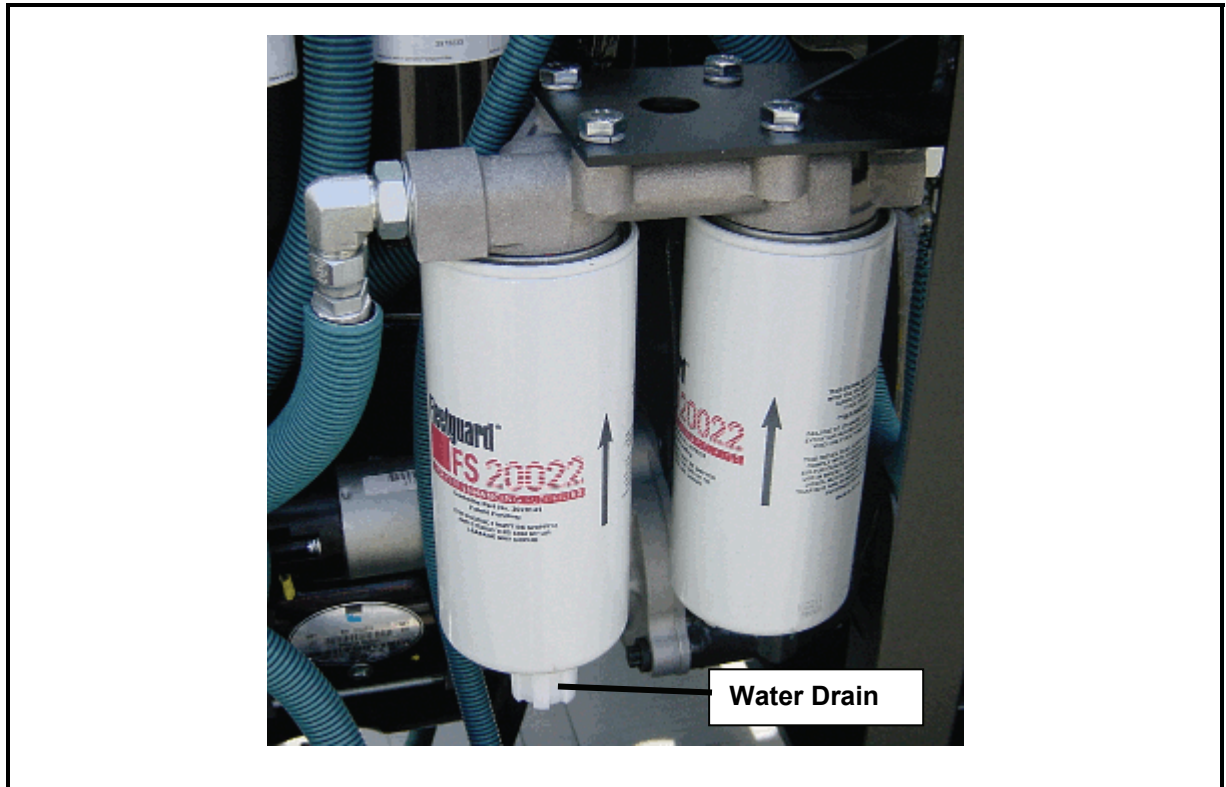
Engine Lubricity Additive Fuel Filters Figure 3
