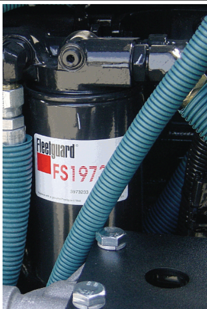
Fuel Water Separator Element (286897-033)
