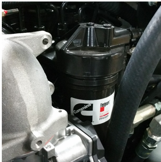
Figure 2-2-6: Primary Fuel Filter
