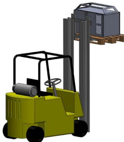
Fig. 4.3.3 Transport and mounting of the AXA2400 by means of a fork-lift truck
