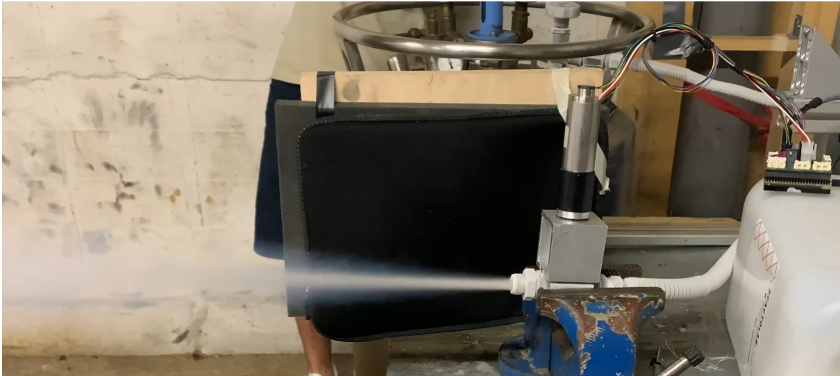
Figure 7.7 – LN 2 leaving the valve.
