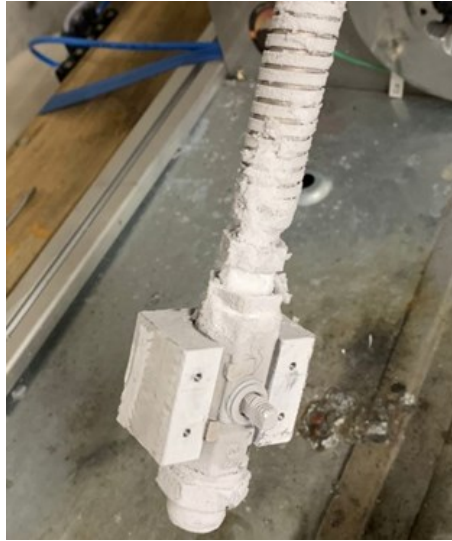
Figure 3.2 - Frozen valve after being connected to LN 2 for 10 minutes.
