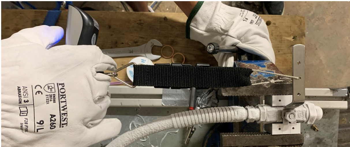
Figure 7.6 – Frozen valve installed in the vise.
