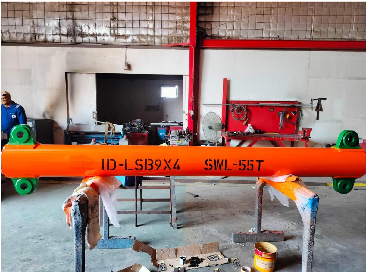
June 2024 – Spreader Beam. Safe Working Load of 55 Tons supplied complete with slings and shackles. Note pad eyes colour coded to the current requirements at time of delivery.
