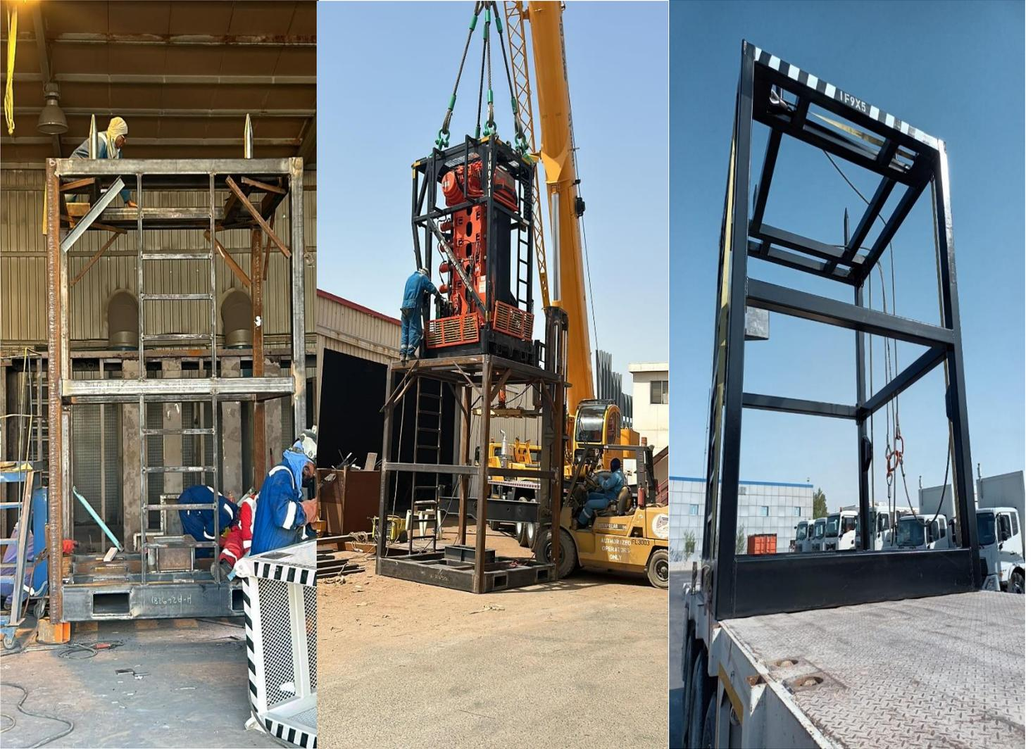
JUNE 2024 – On top priority basis this INJECTOR FRAME FOR OFFSHORE use was fabricated within a very short timescale, including trial assembly of the injector unit to ensure perfect fit up.
