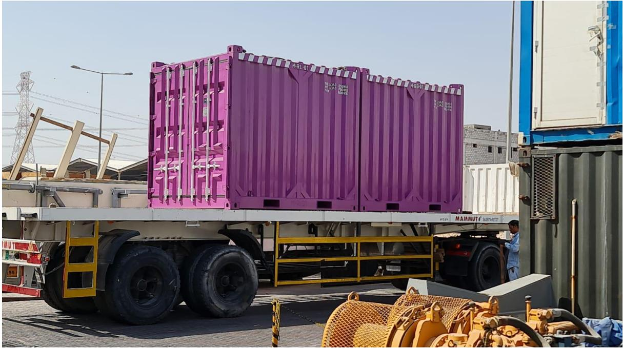
Rigging loft container along with storage container of same size being delivered to our client. Both units were designed to comply with DNV2.7-1 and local requirements for Qatar Energy and NOC.
