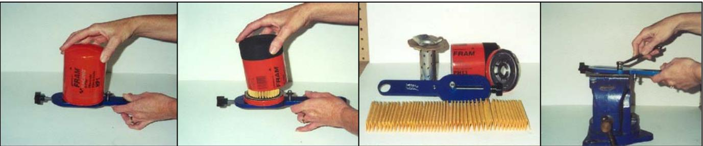
7. Filter element can be inspected by eye or using a magnifying glass.
