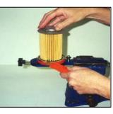
1. Place Oil Filter Cutter (OFC) in vise.
