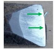
picture to the left. These burrs are very fine, thinner than tin foil and need to be removed before using the tool. If left on, they will fold back upon themselves effectively dulling the edge.
