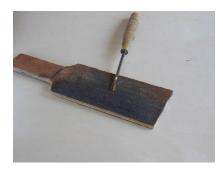
Burrs are removed by stropping, but because they are so fine, they tend to bend out of the way. For this reason, you need to strop the inside edge too and repeat the cycle until the burr has been removed. Alternatively use a buffing wheel.
