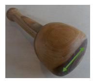
If you look carefully at the mallet on the left, you can see the grain pattern forming a ring. This is indicative of the grain running parallel to the rings as indicated in green. The 'side' grain is weak by comparison with the densely packed 'end' grain. Repeated striking on the side grain will shorten the life of the mallet. The mallet should be used so that the end grain is used to strike the chisel. This will extend the working life of the mallet.
