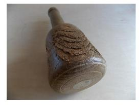
This final picture of a mallet which has seen better days, illustrates what happens if mallets are used for too heavy work and the strikes are taken on the side grain. The grain direction is clear on the mallets head, and the repeated striking on the side grain has caused the grain's strength to fail and the layers have begun to delaminate.
