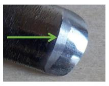
Only a couple of quick rubs will scratch the polish off the surface and prove where the honing has been applied. Here (done deliberately for demonstration) the honing was away from the cutting edge and therefore quite ineffective. Correct this by lifting the handle slightly and repeat. Those with sharp eyes will also note that by rotating the chisel as I rubbed I covered the entire width of the chisel but I was a little light on the bottom edge. More practice needed!
