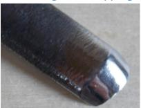
Start by examining your cutting edge. This one is fine and good to use, but I shall use it for demonstration. Note the shine of the stropped (polished) edge. By keeping the edge polished as here not only cuts cleanly but has the following invaluable use.
