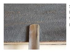
Start the stropping by using the same technique mastered in the honing stage, but on a leather strop. You can check the progress by examining the polish. 8 to 10 rubs in both directions with a rotation should be sufficient to bring the polish finish back.
