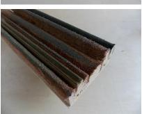
The inside of the chisel requires stropping too. Here strips of wood have been shaped to fit the sweeps of the chisels, then a piece of leather glued to the surface.
