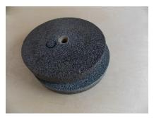
Grind stones, preferred by others, also come in a selection of grits. Here are course and medium grit stones. The finer the stone the quicker it will over heat the cutting edge. Do not use coolants around electric machines unless they have been specifically designed for the purpose. Water cooled grind stones are available but more expensive.
