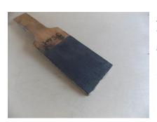
An inexpensive and versatile option for honing is to use a homemade paddle with 'wet and dry' abrasive paper. Here 1200g the abrasive paper has been glue to a piece of plywood, some people prefer to use sellotape, making the paper easier to replace. This abrasive paper can be applied to a piece of dowel as a substitute to a slip stone.
