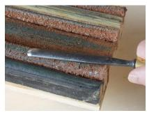
Finish by pulling the chisel over the profile strop to polish the inside edge.
