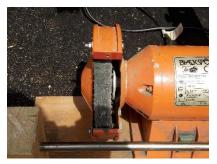
The buffer pad, with a little honing compound, can be used to strop the edge. Here hold the chisel against the rotation buffer pad while pointing down. On another machine: check the direction of rotation before use.
