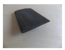
Whenever grinding or honing a chisel, or creating an inside bevel, the inside of the chisel's sweep will become rough or burred. These slip stones are designed for use inside the sweep. They are available in various widths, sweeps and grits.
