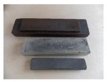
Traditional oil or wet stones can be used, without risk of overheating. They are available in many forms and qualities and of different level of abrasiveness, however for grinding this is slow.
