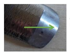
Raise the handle to place the honing on the cutting edge and repeat the above step. Just 4 or 5 rubs in each direction and the honing is complete. The polish is replaced by the dull honed finish right to and across the cutting edge.
