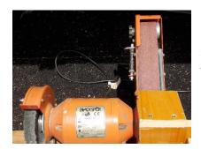
I prefer the belt grinder to the traditional disc or stone grinders because the point of contact with the tool is flat and leaves a flat grind, where stones leave a convex grind. Belts are available in course (80 grit), medium (120 grit) and fine (180 grit).
