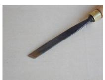
The flat No.2 skew chisels is used to cut into acute corners.
