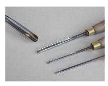
No. 9, 10 & 11 chisels are also called flutters. The very fine chisels are also called veiners. As mentioned above these gouges are the work horse removing most of the waste wood without splitting the wood as well as for detail work such are hair.
