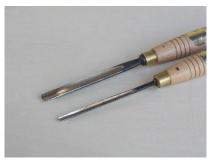
The No.8 chisel is special. All the sweeps are taken from arcs of various circles but with the No.8 the centre of the circle is concurrent with the central axis of the chisel. This means that if you rotate the chisel it will cut a circle. This is particularly useful for carving a sphere e.g. berries and animal eyes.
