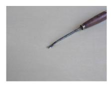
The back-bent chisel is an inverted spoon chisel used in tracery work, and flower stems. Just as the spoon chisel they too are available in a wide range of sweeps and widths.
