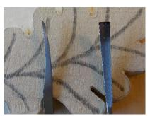
The grounding chisel is also designed to finish the flat, awkward area of the work. Popular for relief carvings. Unlike the foot chisel above the grounding chisels cut at a steep angle allowing access into tighter corners. They also come in a range of sweeps; these are No. 3.
