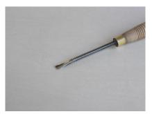
Many of the Sweeps No.1, 3-8 above are also available in the fishtail style. These chisels with their narrow shanks allow access into awkward corner of work. But due to their design with the short body of their cutting section, their useful working life is short lived and where possible I recommend using a normal chisel when access is not restricted.
