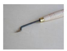
The foot chisel is designed to finish the flat, awkward to access areas of the work. I have recently purchased this tool and yet to try it. Watch this blog for further updates!
