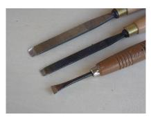
The flat No.1 chisels is ground with a bevel on both sides, and is used centrally to the body. Their sharp, square corners catch on the woodgrain and make it unsuited for finishing. It is particularly useful in lettering. Like most chisels they come in various widths and styles. In the picture, from the top, there is a bull nose chisel, a straight chisel and a fishtail chisel.
