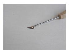
The hooked-skew chisel is in effect the missing number from the fishtail style; being a 'fishtail' for the No.2 chisel. When first used many carver get small cuts until they become familiar with the tool. Handle with care.
