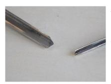
The V tool, named after the 'V' shaped cutting edges, or parting chisel is made by forging two straight carpenter chisels together to form an angle. The angles vary typically 45°, 60° and 90°. There are two styles of parting chisels those with a rounded heel and those with a sharp heel. The latter are more expensive to manufacture and are becoming less common.
