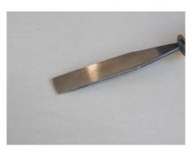
The No.3 & 4 chisels are the first chisels to have any curve to their edge, this lifts the corners off the face of work allowing the smoothing and finishing of surfaces. They may also be used inverted to make convex cuts.
