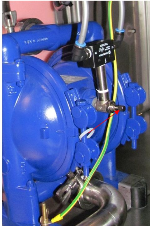
Fig 5.17 adjusting speed of filling/ emptying pump
