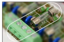
Fuse-protected output: glass fuse
