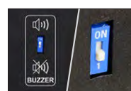
Failure indication - BUZZER
