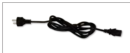
PSD15 Cable 230VAC 3x1mm 2 , 2m, CEE 7/7 (EF), IEC C13
