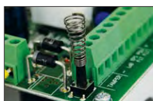
Tamper indicating enclosure opening – 1 piece
