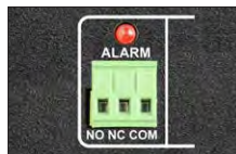
Technical output of failure - relay - NO/NC/COM
