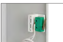
Tamper indicating enclosure opening
