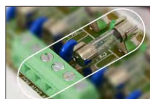
Fuse-protected output: glass fuse
