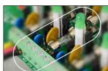
Jumper selectable fuse type: glass fuse / PTC
