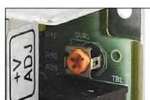
Potentiometer for output voltage adjustment
