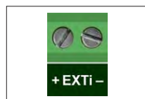
Input of external failure indication EXTi
