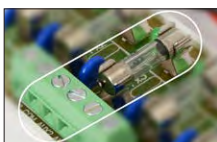
Fuse-protected output: glass fuse
