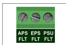
Technical outputs OC type
