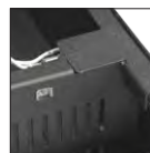
Tamper indicating pulling out of enclosure
