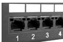
Label field of RJ45 connector
