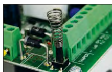
Tamper indicating enclosure opening - 1 piece
