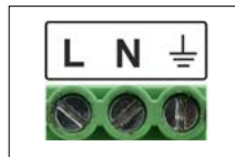
Power input terminals
