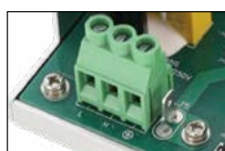
Power input terminals
