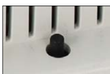
Function START allows running PSU from battery circuit
