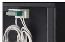
Tamper switch detecting enclosure opening – 1 pcs.
