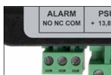
Technical output of failure – relay type – NO/NC/COM
