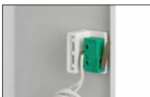
Tamper switch indicating enclosure opening
