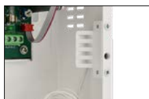
Tamper switch detecting enclosure opening – 1 piece
