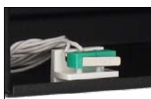
Tamper switch detecting enclosure opening x 2
