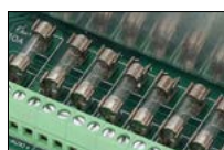
Fuse-protected outputs: glass fuse
