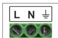
Power input terminals
