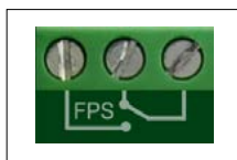
FPS type technical output of fuse failure
