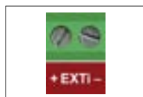
Input of external failure indication EXTi
