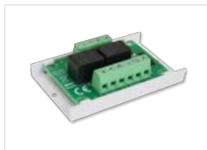
AWZ639 Technical outputs - relay 2x OC → 2x NO/NC/C
