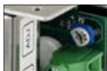
Potentiometer for output voltage adjustment
