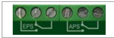
Technical outputs (relay type)
