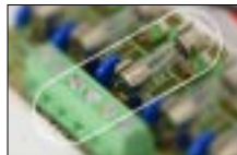
Outputs protected by fuses
