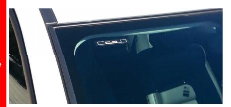
With its high performance and high security features, the VENUS Windshield Tag delivers superior read and write performance. It is designed and tuned for use on the glass windshield of the vehicles.
