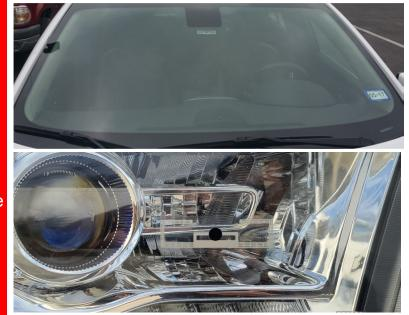
Zenith has been designed as a multi-surface RFID tag. It can be mounted on either a vehicle's windshield or headlamp and is designed and tuned to be a simple, single solu on for any vehicle.
