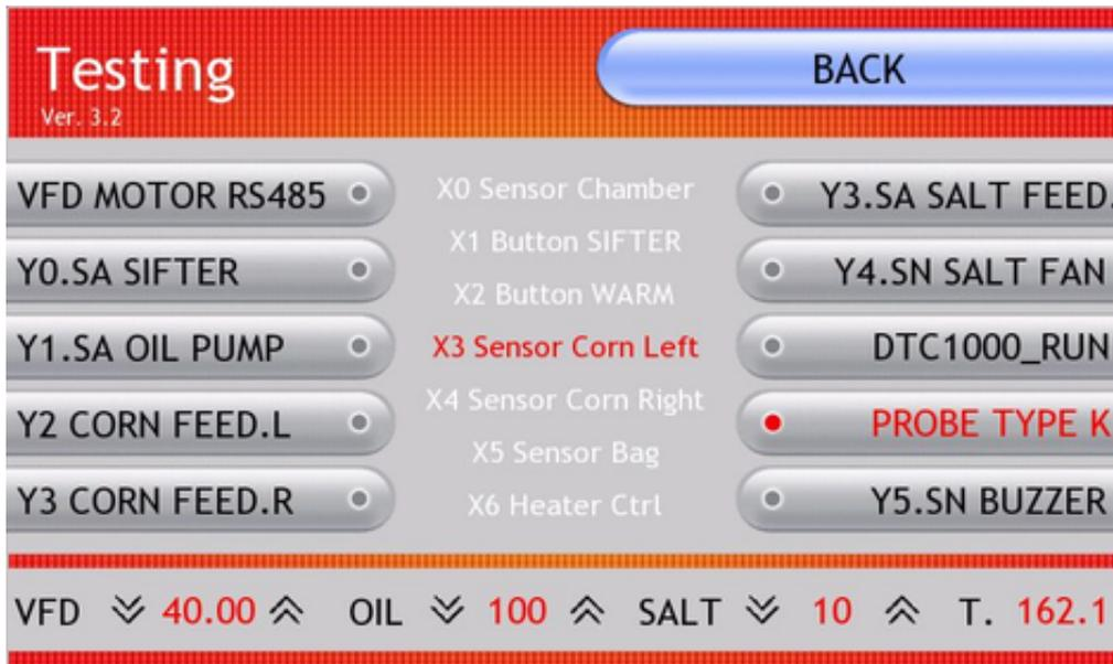
In this screen one can check operation of different parts of the machine, and also see the status of its sensors and so on.
