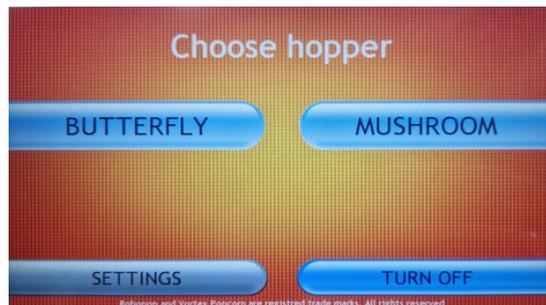
There are two program buttons, BUTTERFLY and MUSHROOM, which allow to run the machine for processing corn from either of two corn bins.
