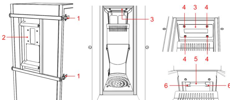
Fig. 6 Light bulb replacing
