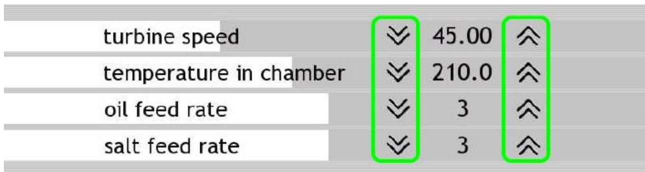
Each type of corn has its own popping temperature. For most kinds of “butterfly” corn the set temperature should be about 210°C, for “mushroom” corn it should be about 220°C.
