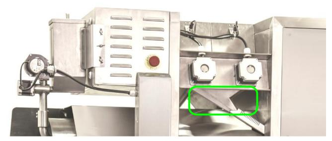
Feed hopper should always be cold because the hopper takes cold air from the outside.
