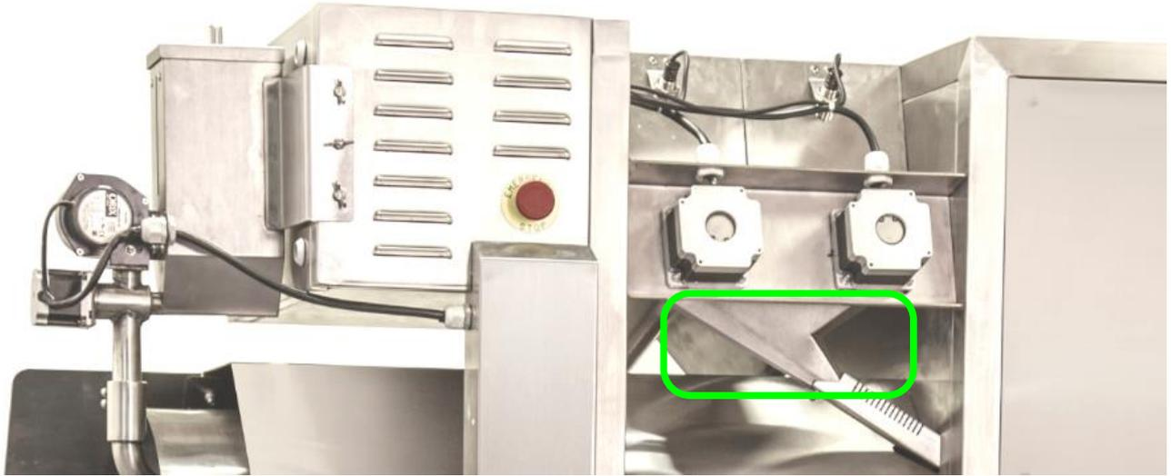
Feed hopper should always be cold because the hopper takes cold air from the outside.
