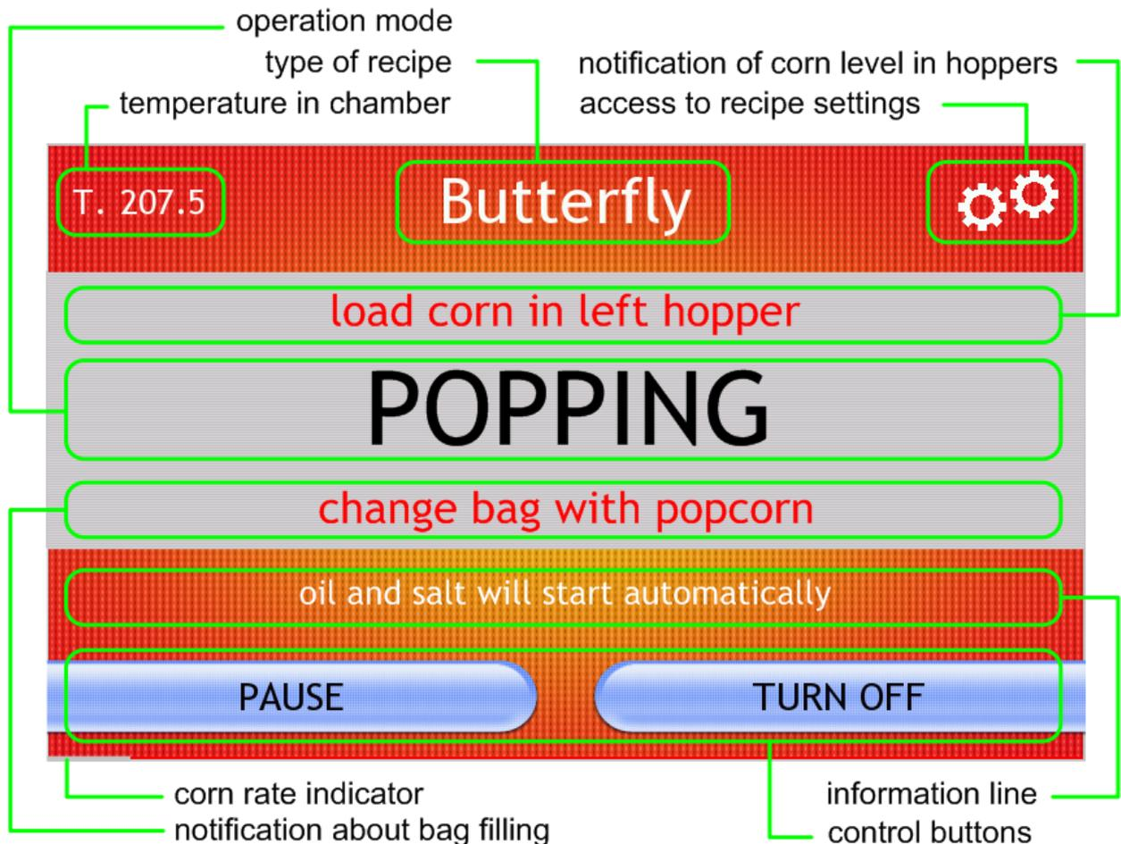
Corn supply begins from the minimum corn speed and gradually increases to the set corn speed. The screen has a white ribbon on the bottom part which indicates the increase of the corn supply. When the ribbon reach the right side it means that the set corn rate is reached. The first popcorn flies out from the chamber in 2 minutes.
