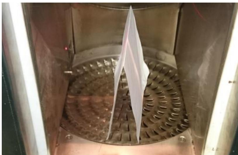
The indicator should turn red. It means that the chamber is overfilled with popcorn.
