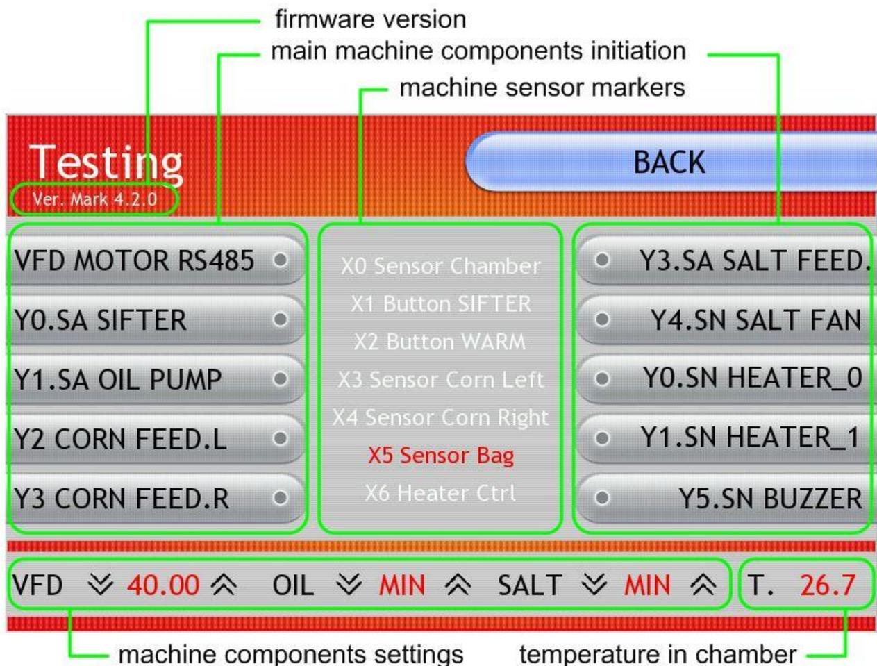
3. Switch on the main motor by pressing VFD\_MOTOR RS485 button. A turbine of the main motor starts to accelerate to the minimal operating frequency. It is 40 Hz. Set 60 Hz by UP
