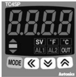
Temperature set point (SV) is 300°C by default. Note that after changing **1n-t** (temperature sensor type) or **Un-t** (temperature unit) values, parameters **H-Su**, **L-Su**, **AL1**, **AL2**, **HY5** must be set again.
