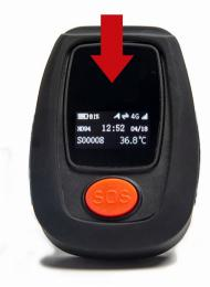
The screen will light up and display the percentage (%) of remaining battery, cell signal strength, and the current date. The G-SAFE is now ready for use.
