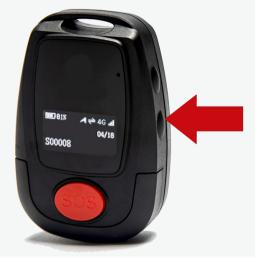
Shutting off the G-SAFE: At the end of the shift, shut off the G-SAFE. Press the bottom button on the side until you hear a beep and vibration. Then connect the magnetic USB cable behind for charging.
