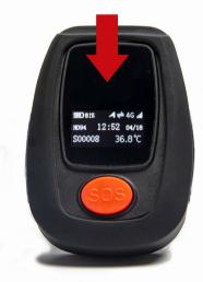
The screen will light up and display the percentage (%) of remaining battery, cell signal strength, and the current date. The G-SAFE is now ready for use.
