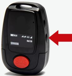
Start the G-SAFE: Press the bottom button on the side until you hear a 'beep' and feel a vibration
