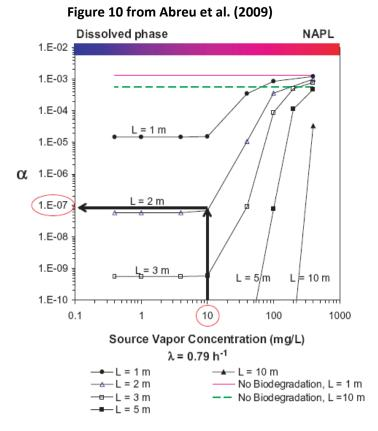
Figure 10. Use of the chart to select a semi-site-specific attenuation factor. For a source concentration of 10,000  $\mu$ g/L and a source-building separation of 2 m, the attenuation factor would be about 1E-7.
