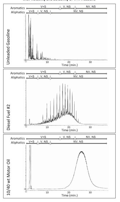
Figure 13-4: GC-FID Chromatograms for Unleaded Gasoline, Diesel Fuel #2, and Motor Oil with Volatility and Solubility of TPH Fractions
