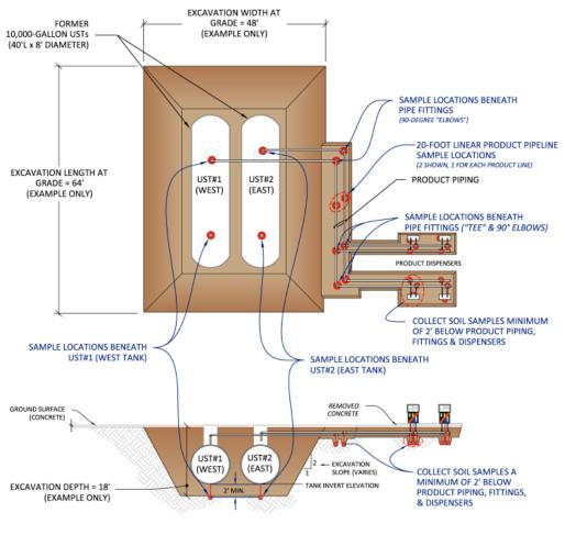
Figure 12-1: Diagram of Tank Removal Soil Sampling: Water Is Not Present
