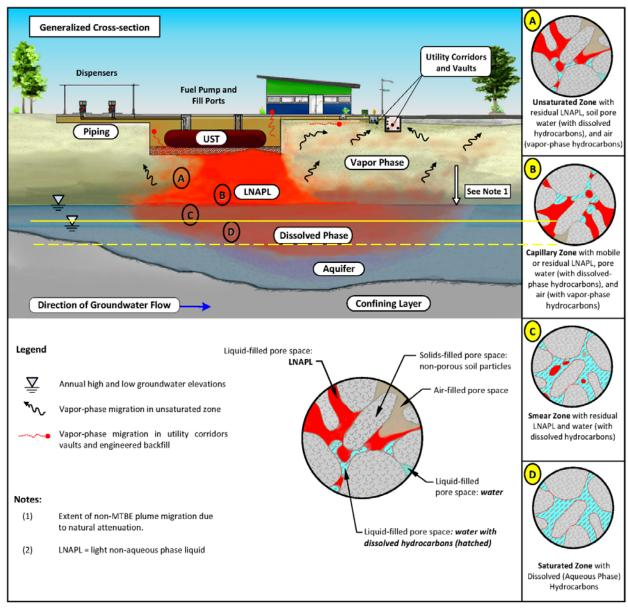
Figure 13-6: Vertical and Horizontal Distribution of Hydrocarbon Phases
