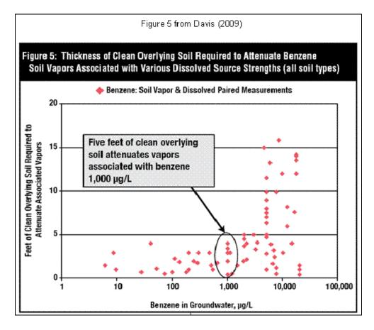
It is important to note in Figure 5, that the exclusion distance (and vapor intrusion risk potential) is relatively independent of the benzene source concentration over the approximate range of dissolved phase concentrations up to  $6,000 \,\mu\text{g/L}$ . The development of more conservative groundwater
