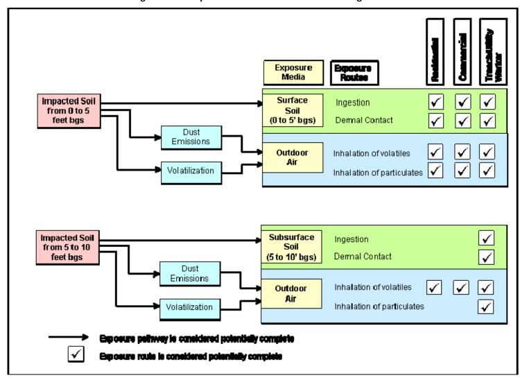
Figure 1. Conceptual Site Model for the Soil Screening Levels.
