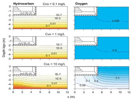
Figure 3. Effect of low vapor source concentration (Cvs) on soil-gas concentration distribution and vapor intrusion attenuation factors ( $\alpha$ ) for basement foundation scenarios and hydrocarbon biodegradation rate  $\lambda = 0.79 \ h^{-1}$ . Hydrocarbon and oxygen concentrations are normalized by source and atmospheric concentrations, respectively.
