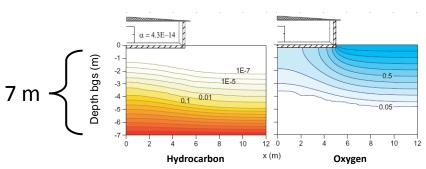
Figure 7. Effect of building type on soil-gas concentration distribution for high vapor source concentration (100,000  $\mu$ g/L) and biodegradation rate  $\lambda = 0.79~h^{-1}$ . Hydrocarbon and oxygen concentrations are normalized by source and atmospheric concentrations, respectively.
