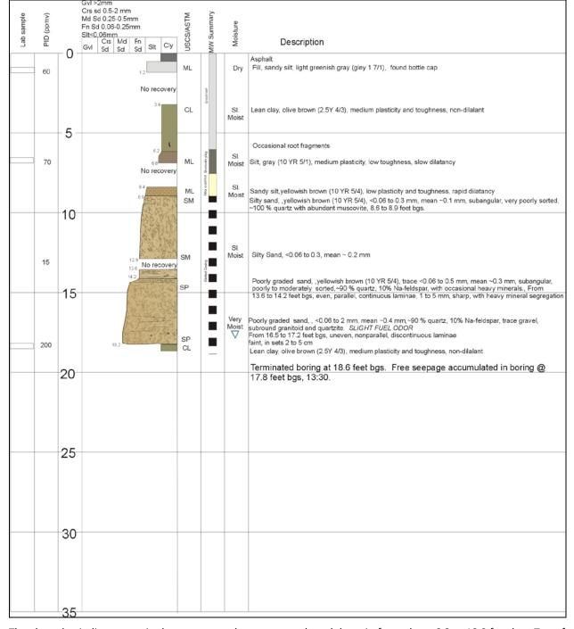
Figure B-1: Example of a Boring Log
