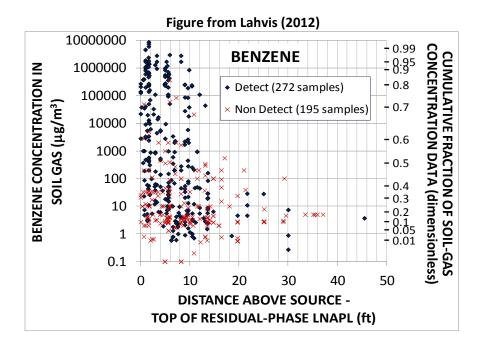
From a conditional probability standpoint, benzene concentrations in soil gas will attenuate below 30  $\mu g/m^3$  at distances of >~ 13 ft above the source in greater than 95% of cases.
