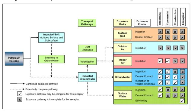
Figure 14-3: CSM Example - After Tank Removal and Observation of Impacted Soil in the Subsurface
