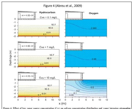
Figure 4. Effect of low vapor source concentration (Cvs) on soil-gas concentration distribution and vapor intrusion attenuation factors ( $\alpha$ ) for slab-on-grade foundation scenarios and hydrocarbon biodegradation rate  $\lambda=0.79~h^{-1}$ . Hydrocarbon and oxygen concentrations are normalized by source and atmospheric concentrations, respectively.
