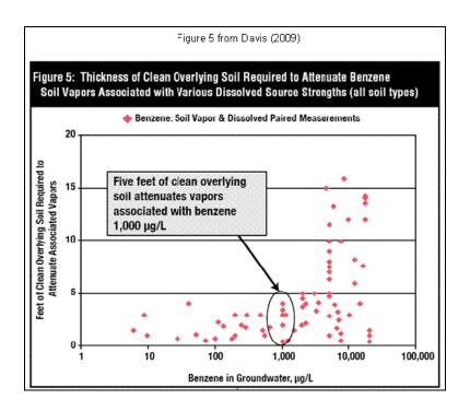
Field (soil-gas) data from Davis (2009) and Wright (2011) show benzene concentrations in soil gas attenuate below 80  $\mu$ g/m³ (see Figure 1) and 20  $\mu$ g/m³ (see Figure 2) within 10 feet above the water table for dissolved-phase benzene concentrations up to 1,000  $\mu$ g/L and 100  $\mu$ g/L, respectively at petroleum UST release sites.
