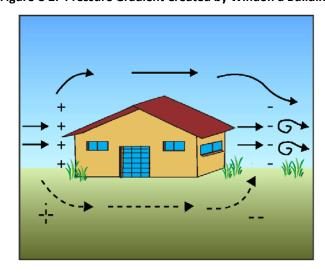
Figure C-2: Pressure Gradient Created by Windon a Building
