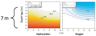
Figure 5. Effect of source depth on the soil-gas concentration distribution and vapor mirusion attenuation factors  $(\alpha)$  for basement scenarios with a high vapor source concentration of  $100,000~\mu g/L$  and biodegradation rate  $\lambda=0.79~h^{-1}$ . Hydrocarbon and oxygen concentrations are normalized by source and atmospheric concentrations, respectively.
