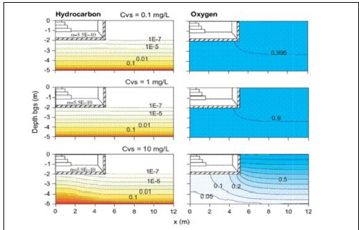
Figure 3. Effect of low vapor source concentration (Cvs) on soil-gas concentration distribution and vapor intrusion attenuation factors ( $\alpha$ ) for basement foundation scenarios and hydrocarbon biodegradation rate  $\lambda=0.79~h^{-1}$ . Hydrocarbon and oxygen concentrations are normalized by source and atmospheric concentrations, respectively.
