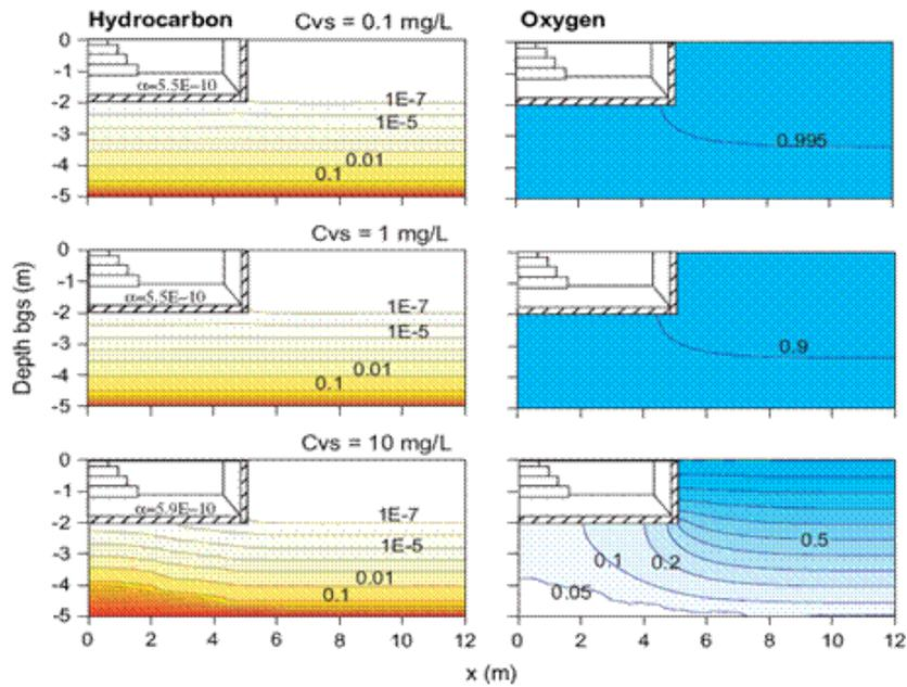
Figure 3. Effect of low vapor source concentration ( $C_{vs}$ ) on soil-gas concentration distribution and vapor intrusion attenuation factors ( $\alpha$ ) for basement foundation scenarios and hydrocarbon biodegradation rate  $\lambda = 0.79 \text{ h}^{-1}$ . Hydrocarbon and oxygen concentrations are normalized by source and atmospheric concentrations, respectively.
