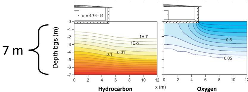
Figure 7. Effect of building type on soil-gas concentration distribution for high vapor source concentration (100,000  $\mu\text{g/L}$ ) and biodegradation rate  $\lambda = 0.79 \text{ h}^{-1}$ . Hydrocarbon and oxygen concentrations are normalized by source and atmospheric concentrations, respectively.
