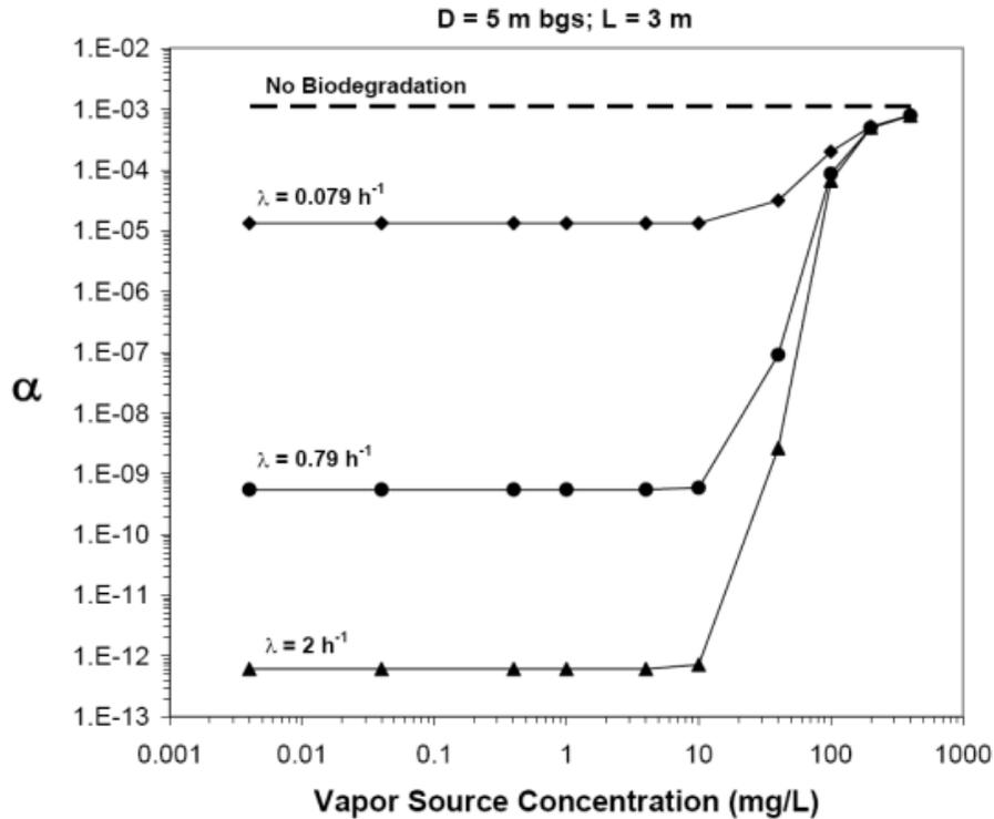
Figure 5—Influence of soil vapor source concentration and first-order biodegradation rates ( $\lambda$ ) on vapor intrusion attenuation factors ( $\alpha$ ) for basement scenarios, homogeneous sand soil and source depth (D) of 5 m bgs (source-foundation separation L = 3 m).
