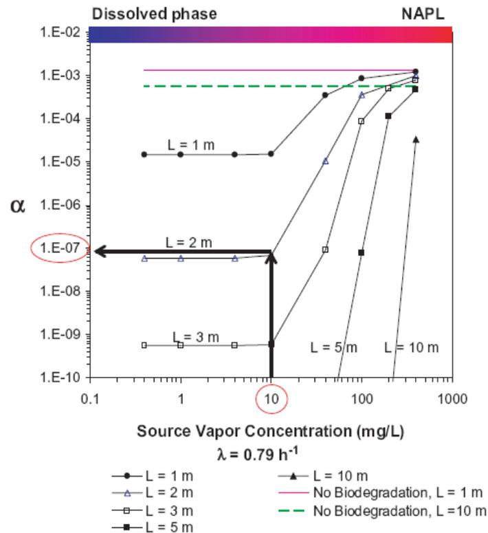
Figure 10. Use of the chart to select a semi-site-specific attenuation factor. For a source concentration of 10,000  $\mu\text{g/L}$  and a source-building separation of 2 m, the attenuation factor would be about  $1\text{E-}7$ .
