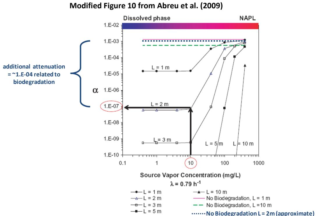
Figure 10. Use of the chart to select a semi-site-specific attenuation factor. For a source concentration of 10,000  $\mu\text{g}/\text{L}$  and a source-building separation of 2 m, the attenuation factor would be about 1E-7.
