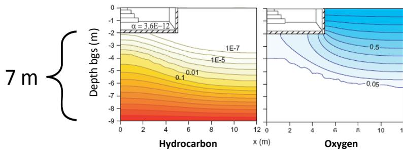
Figure 5. Effect of source depth on the soil-gas concentration distribution and vapor intrusion attenuation factors ( $\alpha$ ) for basement scenarios with a high vapor source concentration of  $100,000\ \mu\text{g/L}$  and biodegradation rate  $\lambda = 0.79\ \text{h}^{-1}$ . Hydrocarbon and oxygen concentrations are normalized by source and atmospheric concentrations, respectively.
