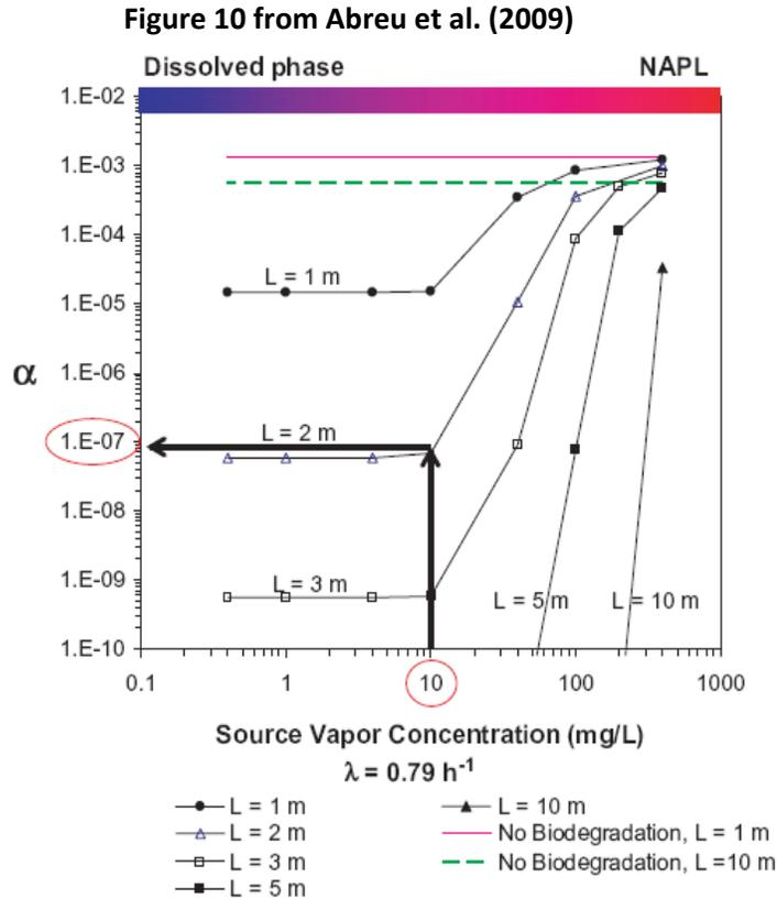
**Figure 10.** Use of the chart to select a semi-site-specific attenuation factor. For a source concentration of 10,000 µg/L and a source-building separation of 2 m, the attenuation factor would be about 1E-7.
